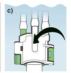
Keeping the endoscope and the distal-end flushing adapter immersed in the water, hold the distal-end flushing adapter and gently pull the endoscope to ensure that the distalend does not come out of the distalend flushing adapter.
