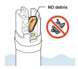
When all debris is removed, put the distal end back in the detergent solution.
