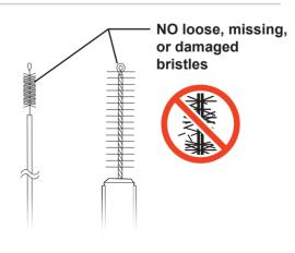
Confirm that the shaft is free from damage.
